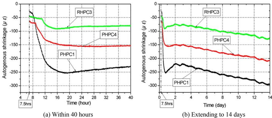
Fig.6. Autogenous shrinkage of HPC specimens within 40 hours and 14 days
