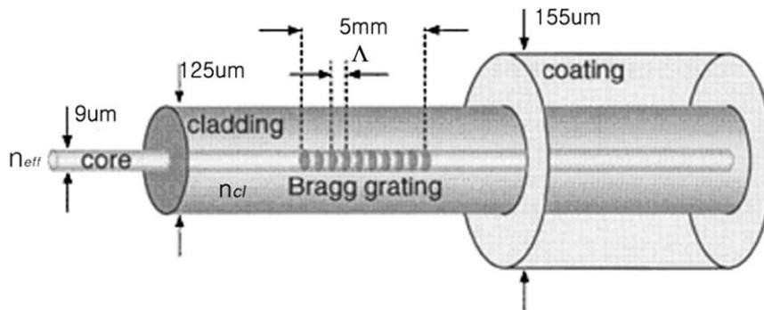
**Fig.1 Schematic structure of a fiber Bragg grating (FBG)**
