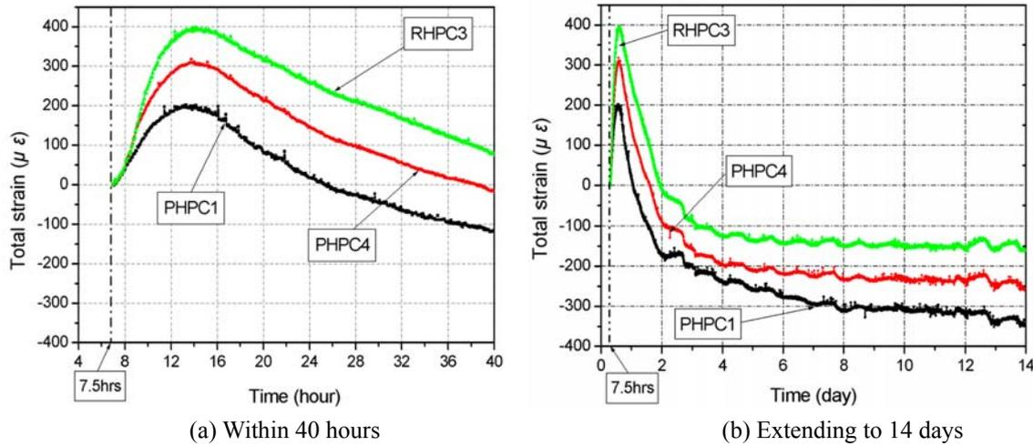
Fig.5. The total deformation of HPC within 40 hours and 14 days
