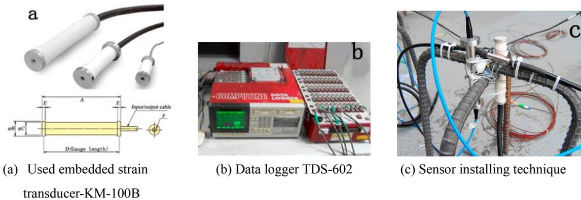
**Fig.3 Used KM-100B strain transducer, data logger and installing technique**
