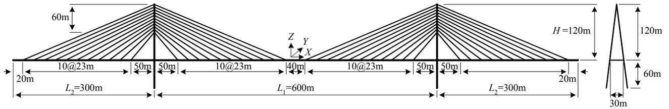
Cable:  $E=200\text{GN/m}^2$ ,  $A=0.01\text{m}^2$ ; Girder:  $E=200\text{GN/m}^2$ ,  $A=0.5\text{m}^2$ ,  $I_y=1.2\text{m}^4$ ,  $I_z=40\text{m}^4$ ,  $J=3\text{m}^4$
