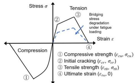
Fig. 3 Stress-strain relations of UHPFRC
