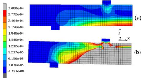
Fig. 5 Principal strain distribution of UHPFRC beam under static at a) initial cracking b) just before failure
