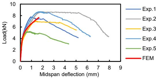
Fig. 4 Evolution of midspan deflection from analysis and experiment.
