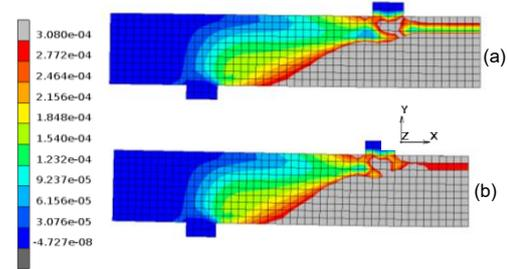
Fig. 8 Principal strain distribution of UHPFRC beam under fatigue (S=0.85) at a) N=1 b) just before failure
