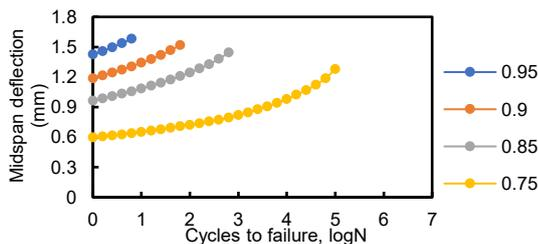
Fig. 6 Evolution of midspan deflection from analysis
