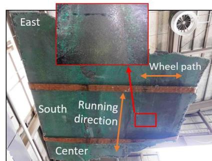
**Figure 5** Interfacial bond layer after removing UHPFRC
