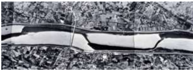
Fig. 1. Alternate bars in the Naka River, an artificially straightened river in Japan. Image courtesy: S. Ikeda. Available: slideplayer.com. 5)
