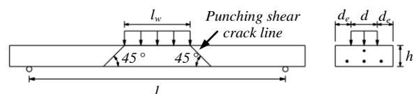
Fig. 2 Geometry of the simplified RC beam and the punching shear cracks
