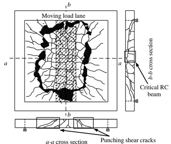
Fig. 1 A typical failure crack pattern of an RC slab under cyclic moving loads
