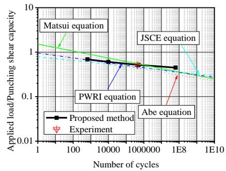
Fig. 5 Fatigue life from different approaches
