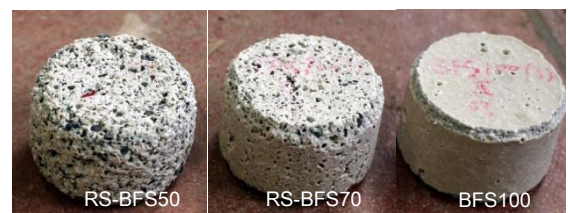
Photo 5 Appearance of specimen after 1 week soaking in the 3% acid solution
