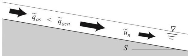
Fig. 2 Conceptual diagram of the normal flow condition without a step, and the definition of  $\tilde{u}_n$
