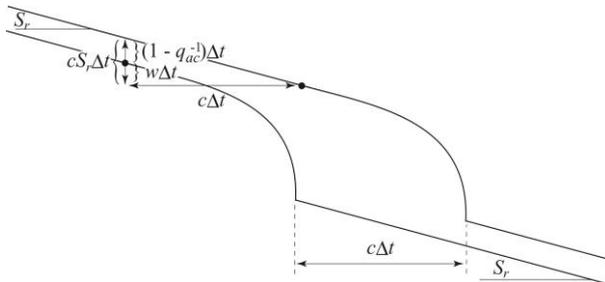
Fig. 4 Conceptual diagram of a permanent form of a step, and the definition of  $c$  and  $w$
