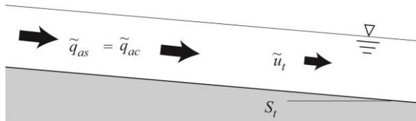
Fig. 3 Conceptual diagram of the threshold condition for bedrock incision, and the definition of  $\tilde{u}_t$
