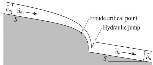
Fig. 5 Conceptual diagram of the flow around a solitary step equation is the definition of  $u_1$ :
