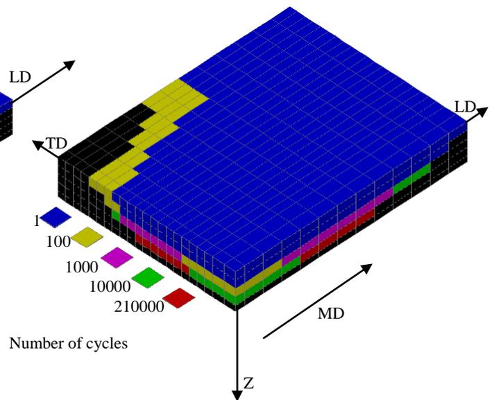
Fig. 8 Propagation of cracked element for slab with frost damage (bottom surface showed on top)
