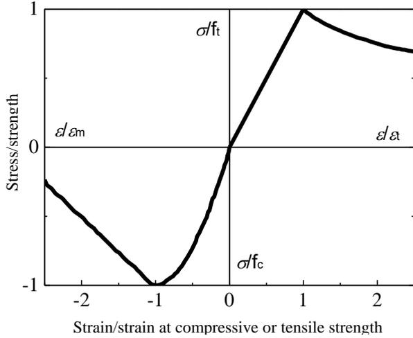
Fig. 1 Normalized stress-strain relationship for concrete
