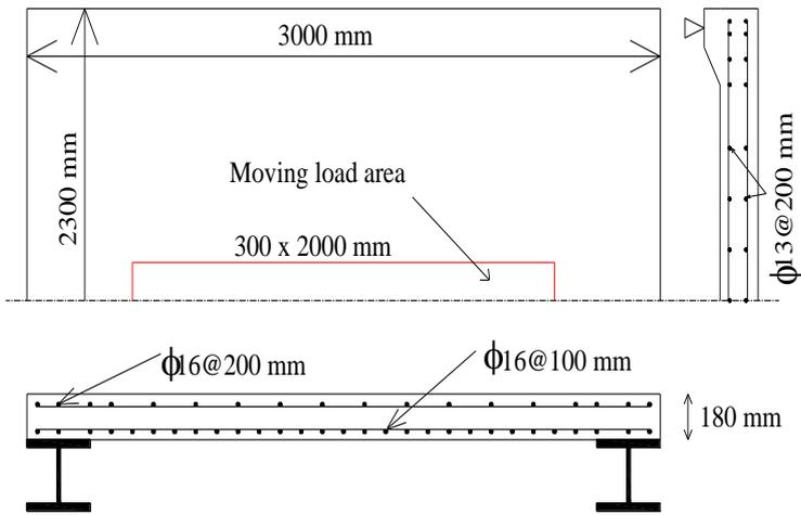
Fig. 5 Slab geometry
