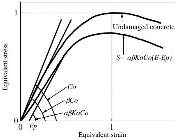
Fig. 3 Equivalent stress-equivalent strain relationship for frost damaged concrete<sup>1)</sup>
