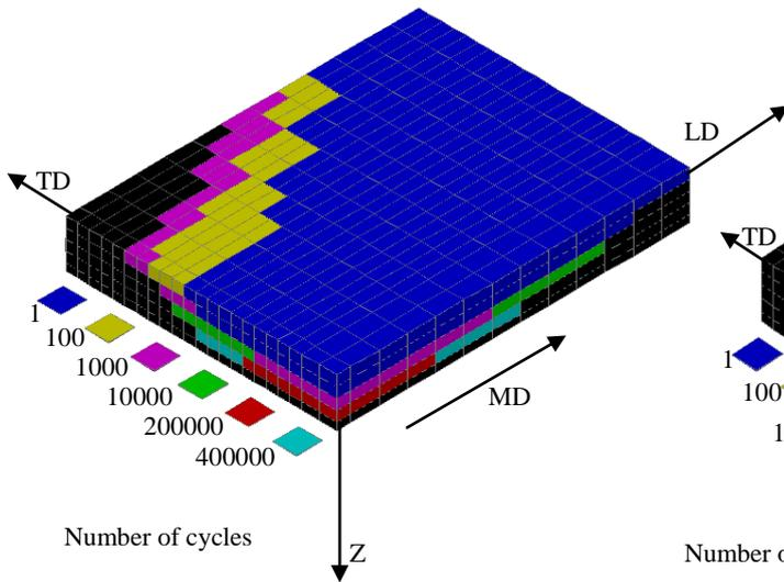
Fig.7 Propagation of cracked elements for slab without frost damage (bottom surface showed on top)
