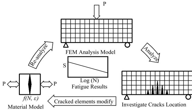
Fig. 1 Scheme of fatigue analysis
