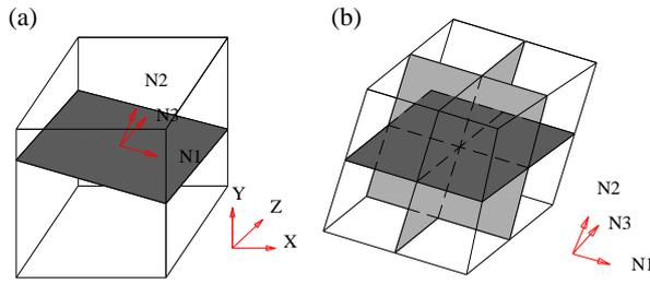
Fig. 2 Crack formation: (a) initiation of first crack; (b) three perpendicular crack formations
