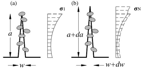
Fig. 3 Crack propagation due to bridging stress: (a) first cycle; (b) after  $N$  cycles
