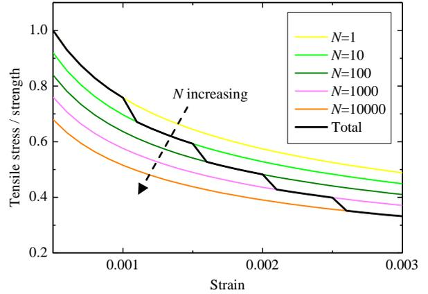
Fig. 4 Crack bridging degradation
