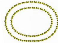
Figure -6 (m,0)=(27,0)/(36,0)の DWCNT 座屈後断面図
