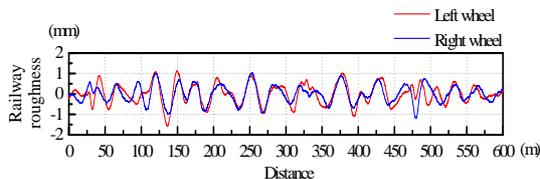
**Fig. 4** Vertical railway roughness
