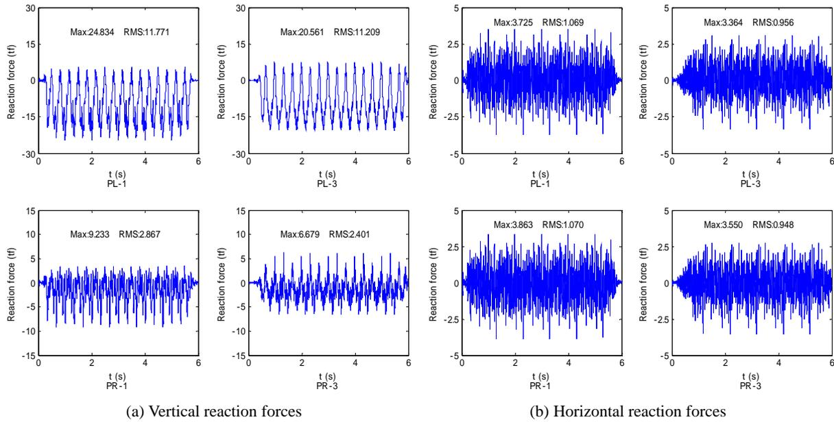
Fig. 7 Reaction forces at the pier bottoms
