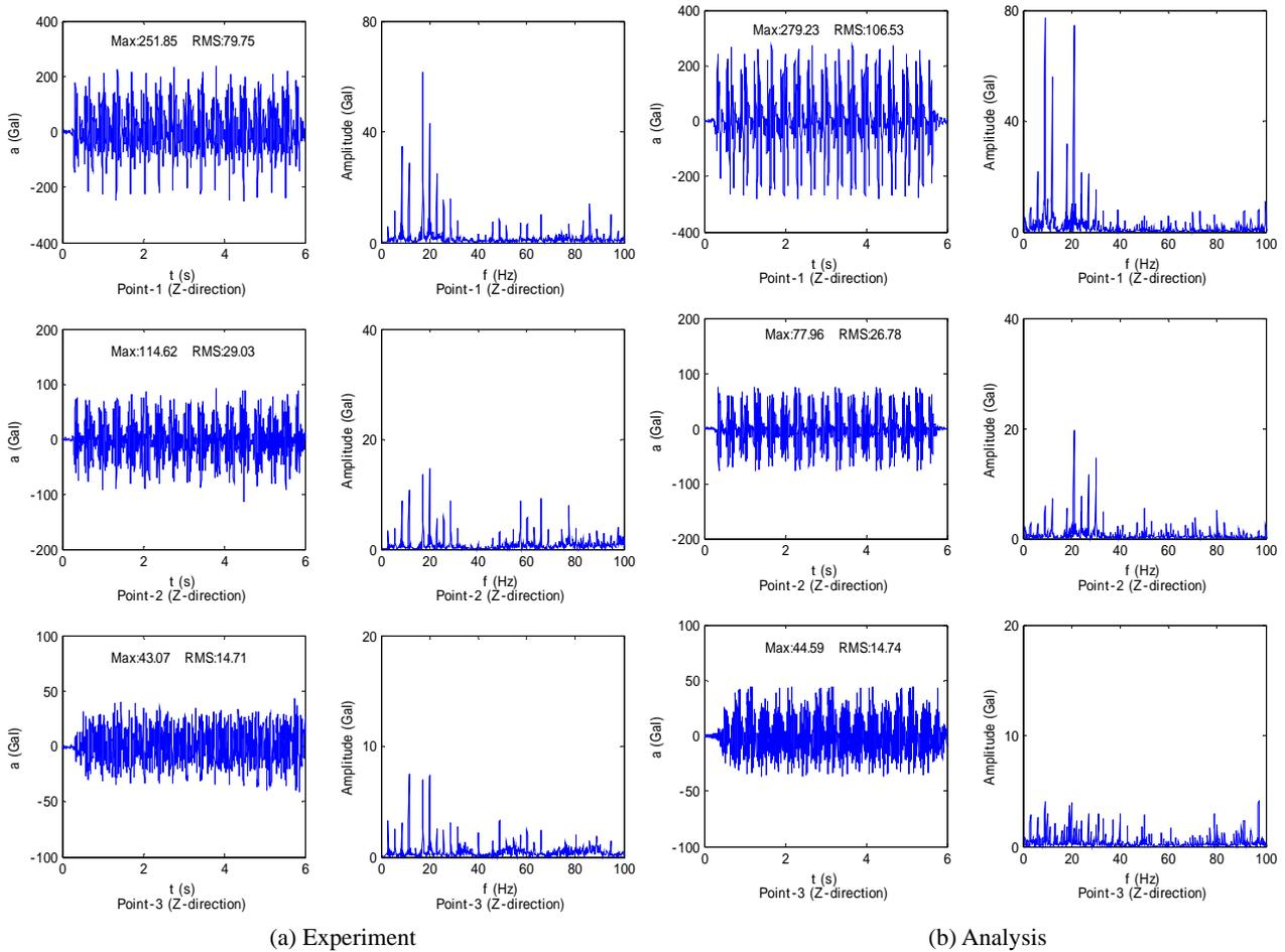
Fig. 5 Vertical acceleration of viaduct
