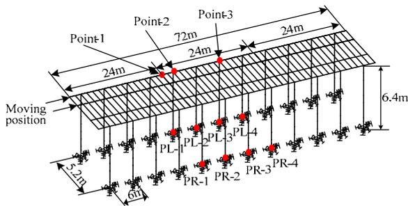
**Fig. 3** Analytical model of viaduct
