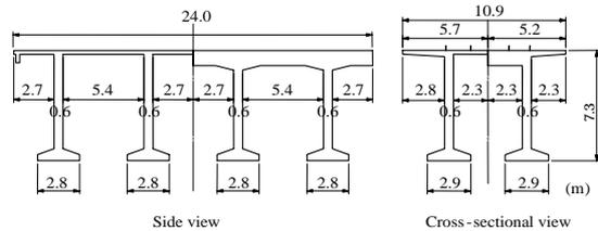
**Fig. 2** Dimensions of viaduct
