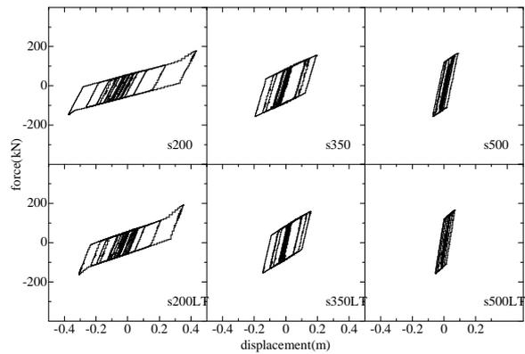
**Fig.5** Shear Force-Displacement Response at Bearing
