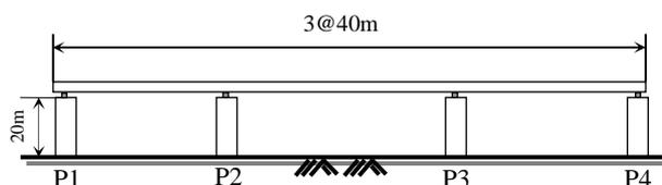
**Fig.1** Three-span Continuous Bridge Viaduct
