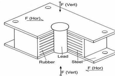
Fig.3 Rubber Bearing with Lead Plug Inside(LRB)
