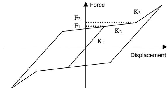
Fig.4 Analytical Model of LRB
