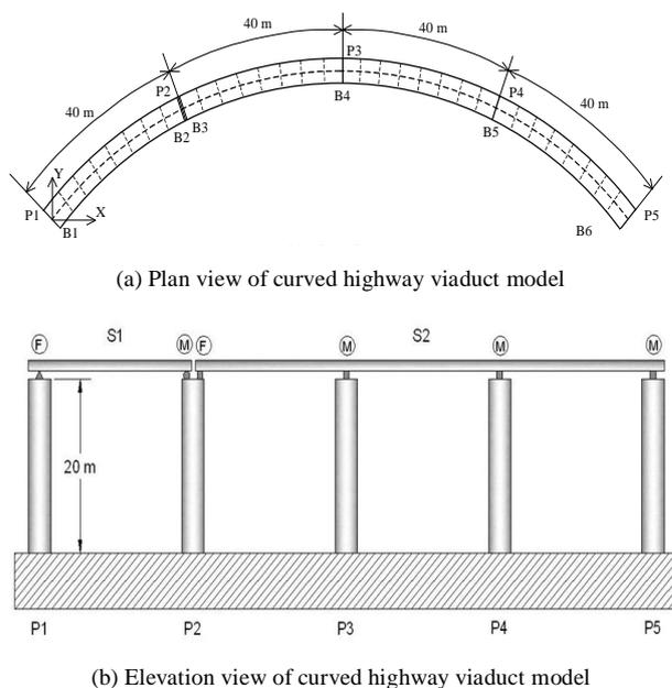
Fig. 1 Analytical model of viaduct
