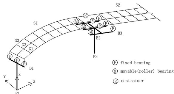
Fig. 2 Detail of curved viaduct finite element model
