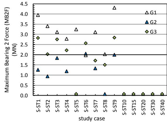
(b) Maximum bearing 2 force in tangential direction
