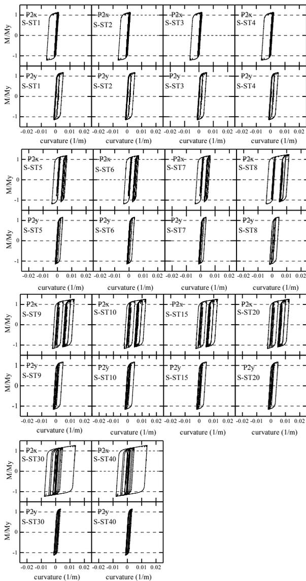
Fig. 7 Bending moment ratio at pier 2 bottom
