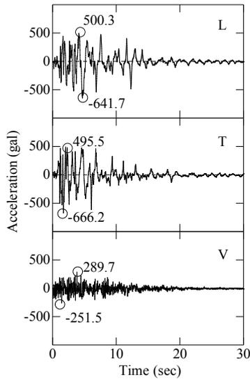
Fig. 4 JR Takatori St. record 1995 Hyogoken Nambu earthquake
