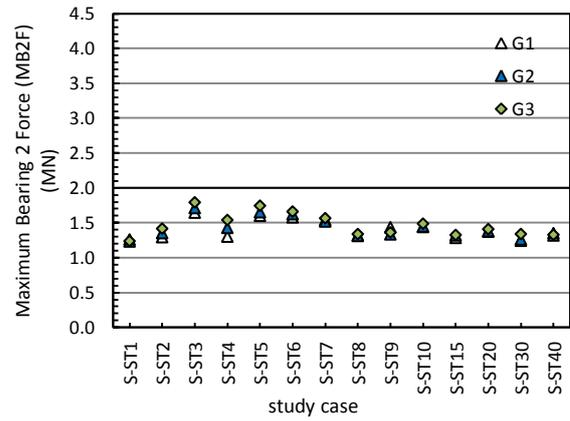
(a) Maximum bearing 2 force in radial direction
