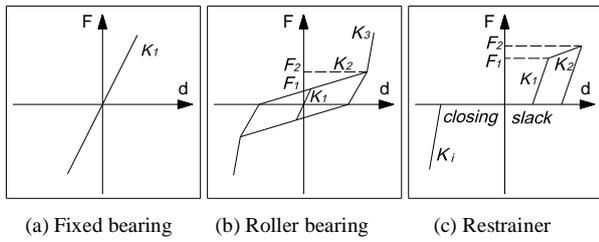
Fig. 3 Analytical models of steel bearing supports and restrainer
