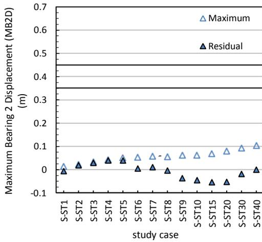
Fig. 5 Evaluation of deck unseating damage for TAK input
