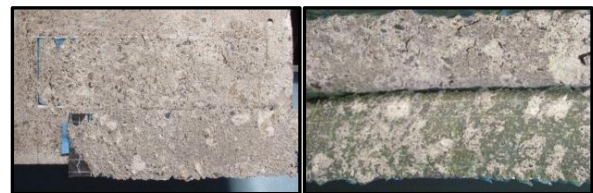
Figure 4 Failure surfaces for E-200 and FP-NS respectively for normal strength concrete substrate
