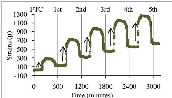
**Fig. 5** 100% saturated mortar strains without thermal effect
