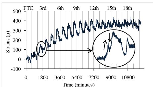
**Fig. 6** 92% saturated mortar strains without thermal effect
