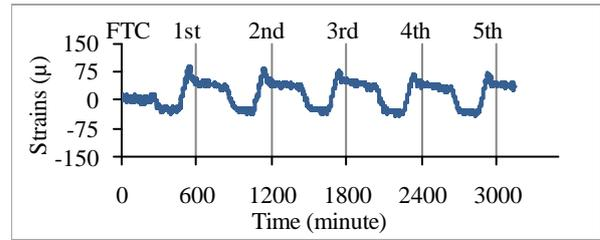
**Fig. 7** 68% saturated mortar strains without thermal effect
