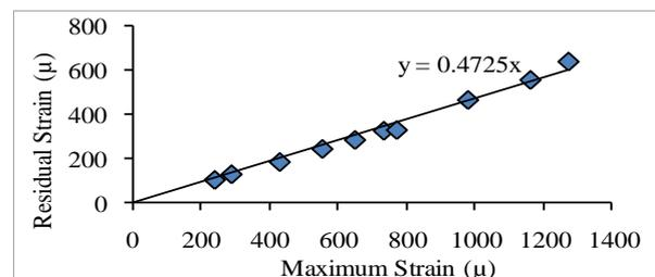
**Fig. 10** Maximum and residual strain relationship
