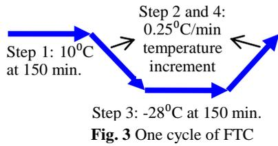
The experiment set-up is illustrated in Figure 2. Specimens were placed inside an environmental chamber to undergo FTC. One temperature history of FTC is shown in Figure 3. This FTC was repeated 5 times for absolutely dry specimens, 100% saturated, and 68.4% saturated while for 92% saturated specimens the FTC was repeated 20 times.
