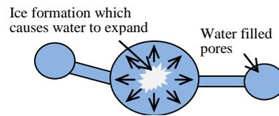
**Fig.8** Pores inside a fully saturated mortar: Ice formation causing large expansion and water filled pores
