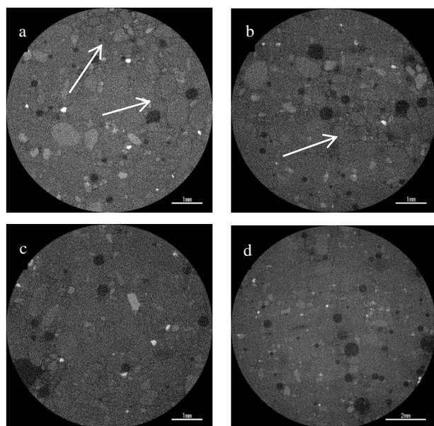
**Fig. 11** 2D images of the internal structure of mortar
