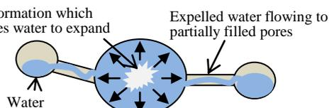
**Fig.9** Pores inside a partially saturated mortar: Ice formation and expelled water flowing to partially filled pores
