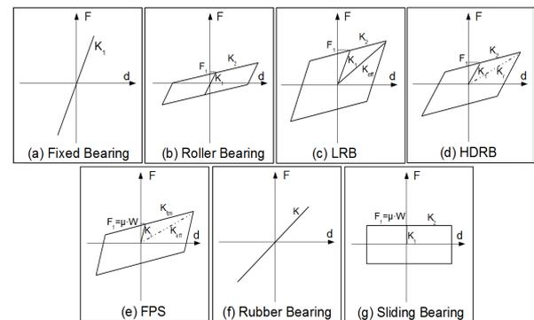
**Fig. 2** Analytical models of bearing supports
