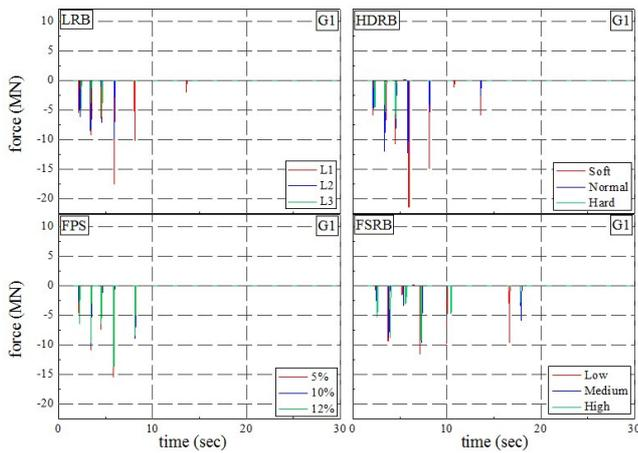
Fig. 3 Impact forces at the expansion joint
