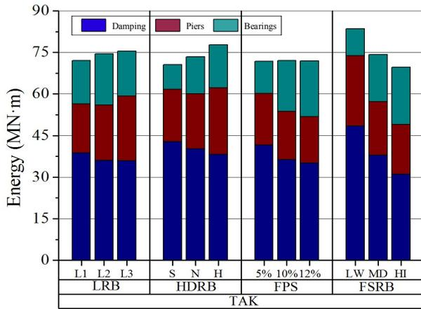
Fig. 6 Energy distribution at the end of the earthquake
