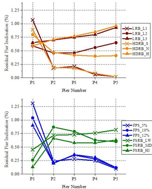
Fig. 4 Residual pier inclination
