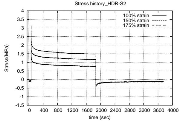
Figure 4. Stress history (HDR-S2) obtained from SR test at different strain levels.
