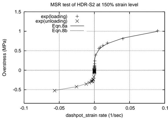
Figure 8. Identification of viscosity parameters
