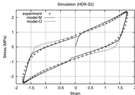
Figure 10. Numerical simulation of 4<sup>th</sup> cycle stress-strain response of basic test
