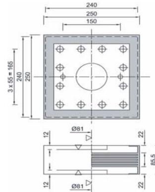
Figure 1. Plan and side view of the specimen
