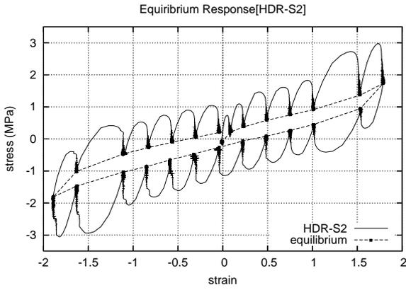
Figure 6. Equilibrium response obtained from MSR test
