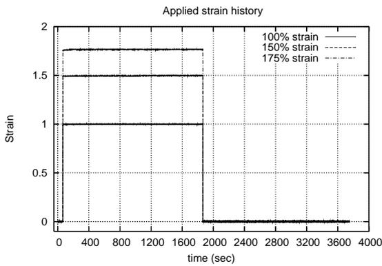
Figure 3. Strain history applied in SR test
