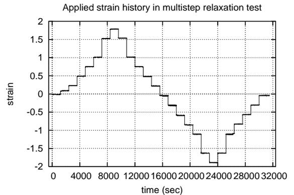
Figure 5. Applied strain history in MSR test
