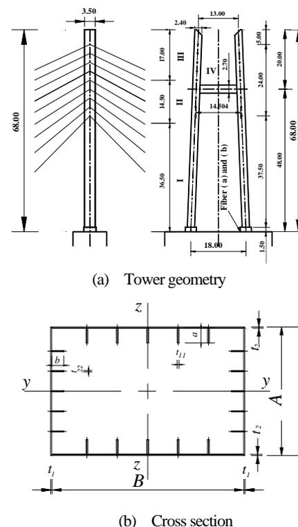
**Fig. 1** Steel tower of cable-stayed bridge
