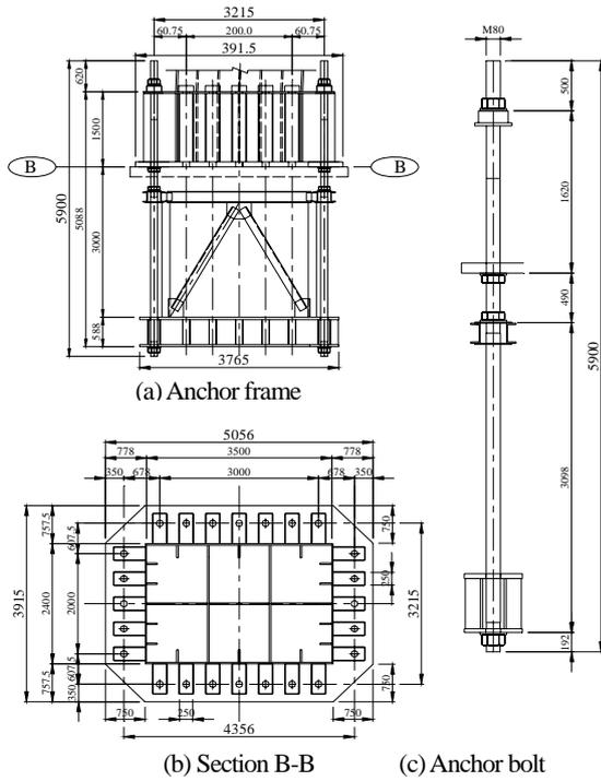
Fig. 2 Details of steel tower base connection (mm)
