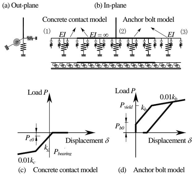
Fig. 3 Base connection components constitutive models
