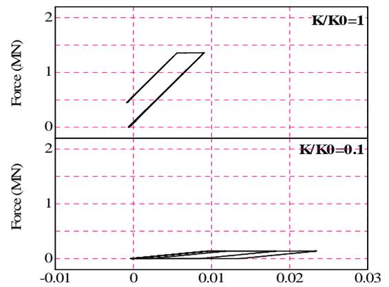
Fig. 8 Anchor bolt load deflection relationship
