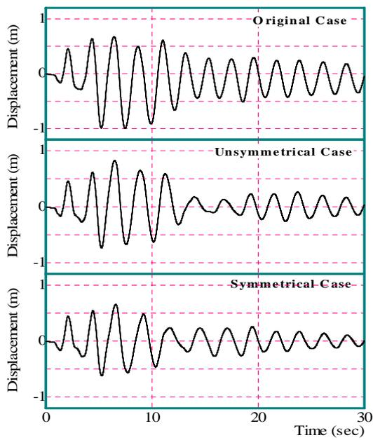
Fig. 5 Displacement time history at tower top
