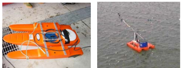
写真-1 ADCP (a) Work Horse (b) Stream Pro
