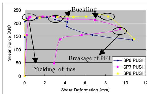
Fig 6. Shear force versus shear deformation
