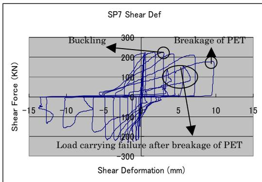
Fig 8. Shear force versus shear deformation SP7
