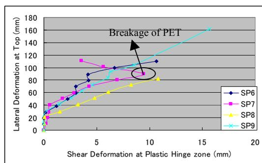
Fig 5. Shear def. versus lateral def.
