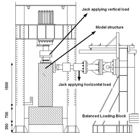
Fig2. Experimental device
