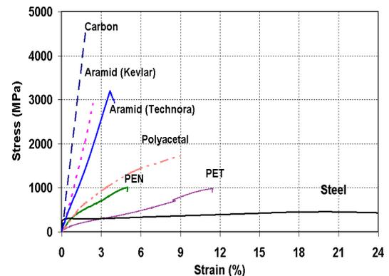
Fig 1. Stress-strain curves for various materials
