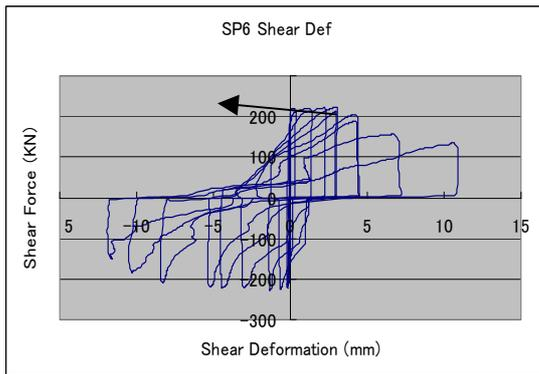
Fig 7. Shear force versus shear deformation SP6
