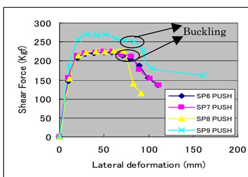
Fig4. Envelope curves of specimen
