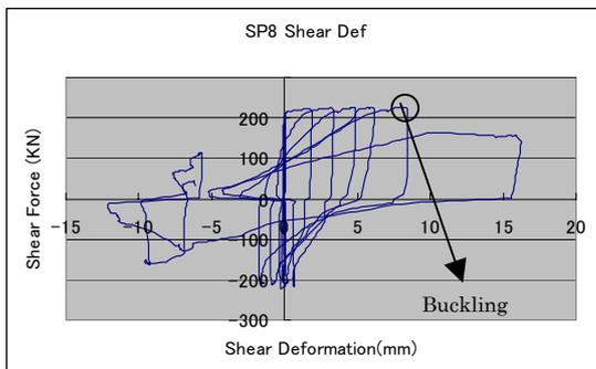
Fig 9. Shear force versus shear deformation SP8
