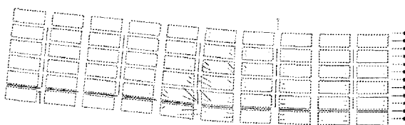
(c) 曲げ破壊先行型-劣化度1-R (F-D1-R)
