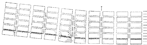
(a) 曲げ破壊先行型-劣化度1-SR (F-D1-SR)
