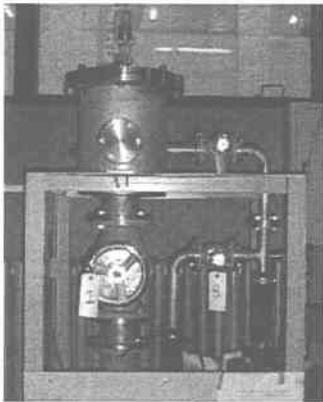
Fig.2 10^{-3}\text{torr} Vacuum Chamber and Pump
