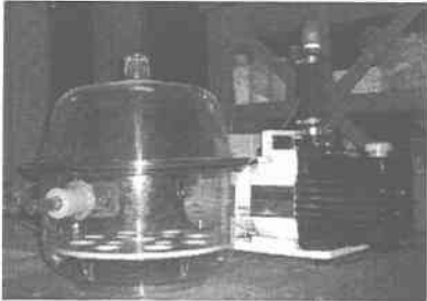
Fig.1 10^{-1}\text{torr} Vacuum Chamber and Pump
