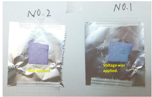
Fig. 7 Paper towels with the anthocyanin and salt solution after drying.
