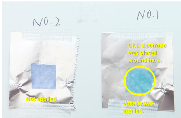
Fig. 5 Comparison between paper towels after absorbing the solution with and without the radio wave irradiation by an RFID reader.
