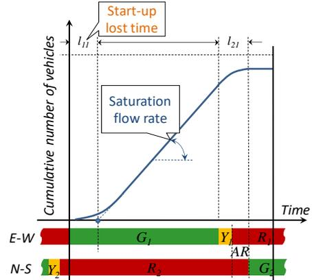
Fig. 2 SLT measurement method
