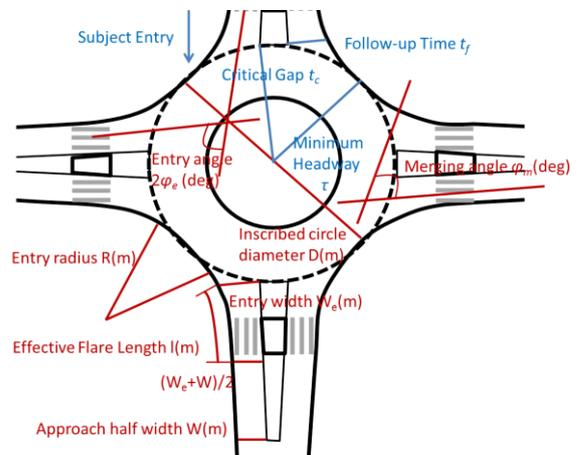
Fig.2 Definition of geometric parameters and cross-sections for measuring gap parameters.
