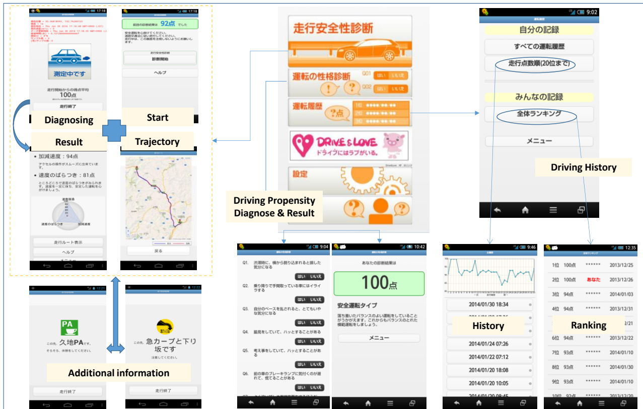
Figure 1. System Design of the App Safety Supporter
