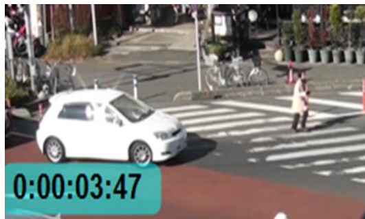
Fig.11: Driver rejected gap safely at modified intersection corner
