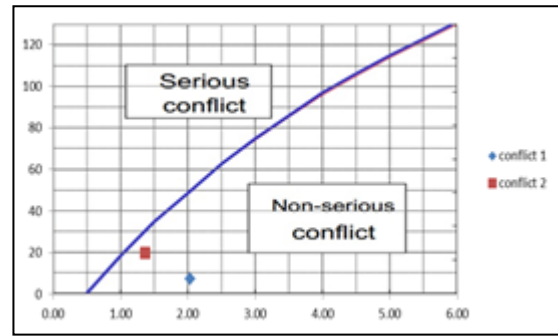
Fig.12: Seriousness of sudden brake which is taken by left turn driver using TA-CS graph
