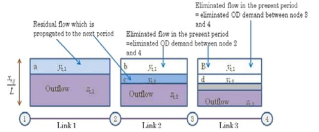
Figure 1. Semi-dynamic traffic assignment model
