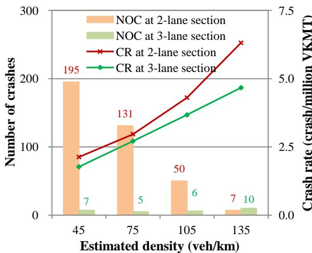
Fig.6 Crash rate-density at basic segment (congested flow)
