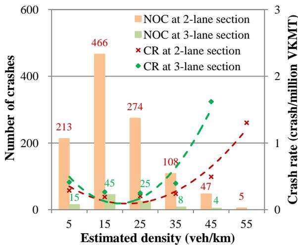
Fig.5 Crash rate-density at basic segment (uncongested flow)
