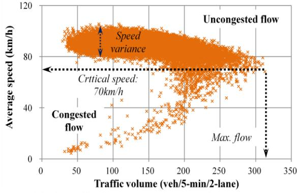
Fig.2 Traffic flow-speed diagram of a bottleneck
