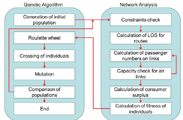
Fig.2 . Flow chart of the Genetic Algorithm
