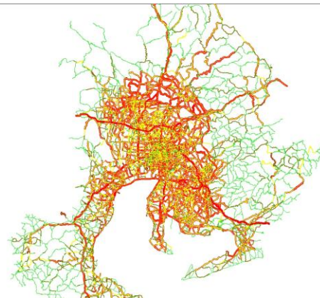
Fig.8 Needed power in network when microcar rate equals 0%
