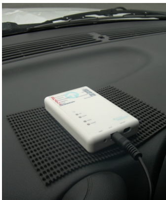
図-2 BCALs設置状況
