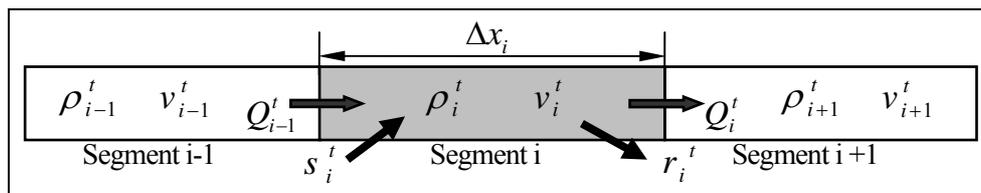
Figure 3 : Discrete model of the freeway section
