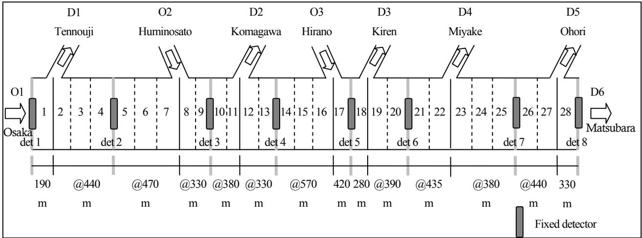
Figure 2: Schematic layout of the road section
