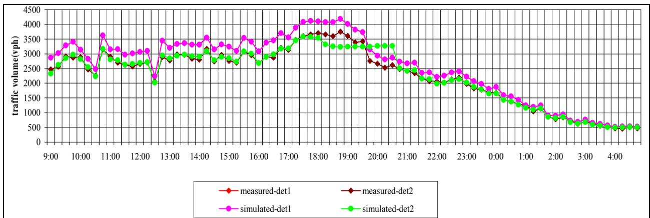
Figure 4: Observed and simulated traffic volumes at detector 1 and 2
