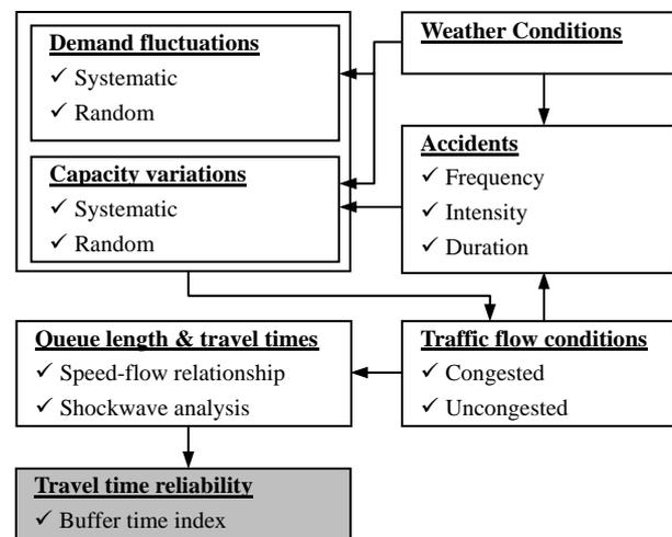
Figure 1: Framework of the simulation model
