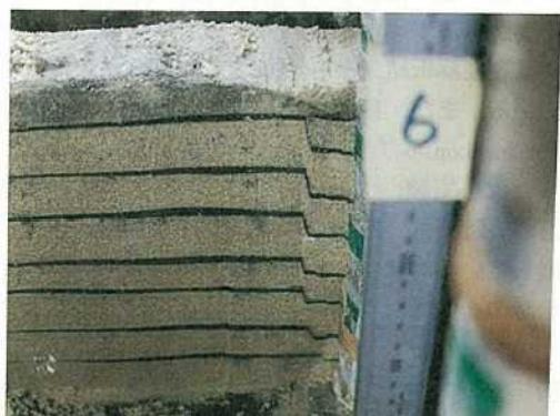
(c) 破壊断面(DSFT-03,Hp=20m)
