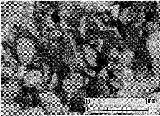
Photo.1 (a) Photomicrograph of Dogs Bay sand
