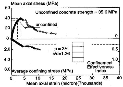
Fig.8 Stress-strain, confinement : s/d=1.26 - specimen J19-225 -
