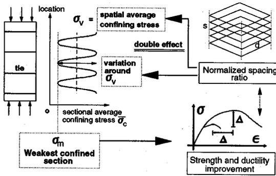
Fig.20 Double effect of  $r/f$  spacing
