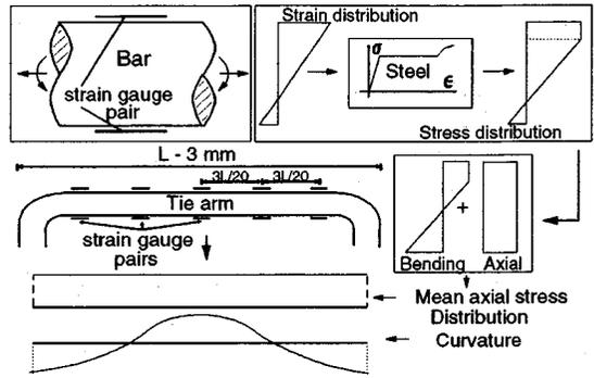
**Fig.3** Spatial stress measurement in lateral r/f
