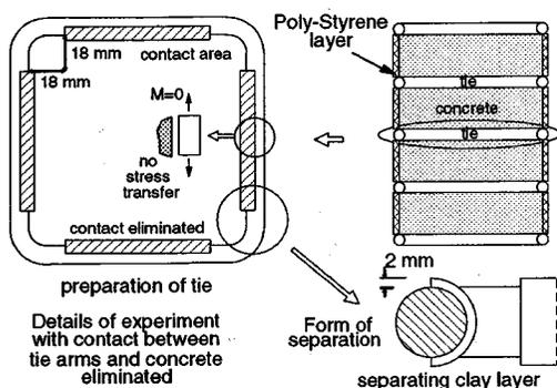
Fig. 12 Specifications for corner action test
