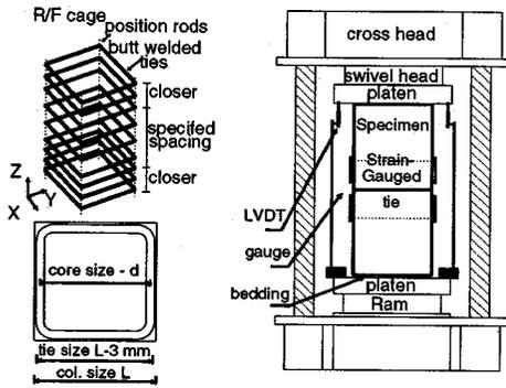
Fig.2 Specifications and experimental setup
