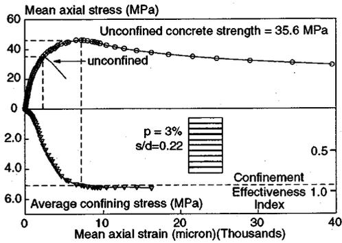
Fig.5 Stress-strain, confinement : s/d=0.22 -specimen A09-042 -
