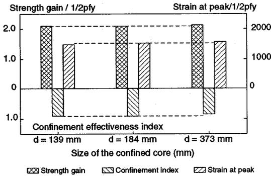
**Fig. 4** Core size effect on confinement
