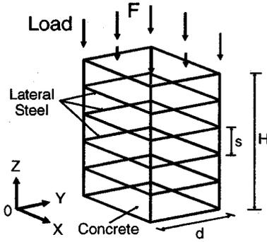
Fig.1 Confined concrete core
