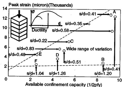
Fig.15 Ductility and potential confining capacity at the peak strength of core
