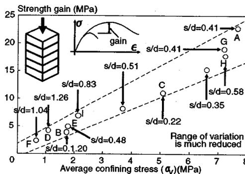
Fig.16 Strength gain with induced average confining stress at the peak of the core
