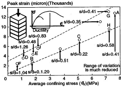
Fig.17 Peak strain with induced average confining stress at the peak strength of the core
