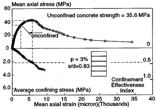
Fig.7 Stress-strain, confinement : s/d=0.83 - specimen I16-150 -
