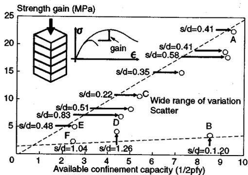
Fig.14 Strength gain and potential confining capacity at peak strength of core
