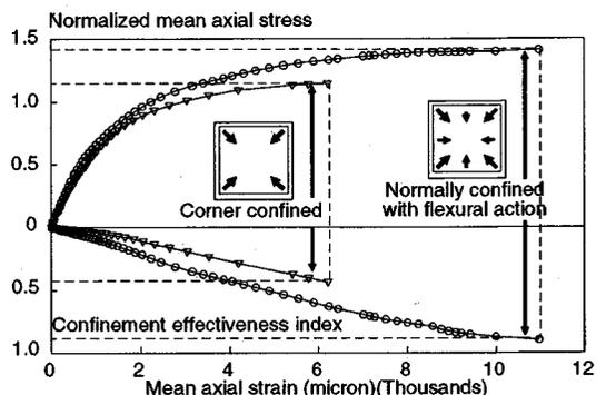
Fig. 13 Stress-strain, confinement for corner and contact actions
