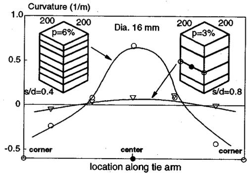
Fig.11 Curvature profiles of the same diameter tie (C16-075 and I16-150 in Table 1)
