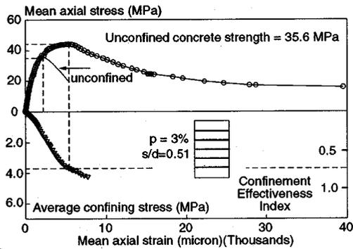
Fig.6 Stress-strain, confinement : s/d=0.51 - specimen H13-094 -
