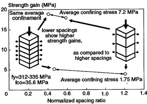
Fig.18 Strength gain under same average confining stress
