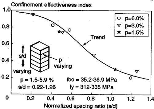
Fig.10 Confinement effectiveness index against spacing ratio
