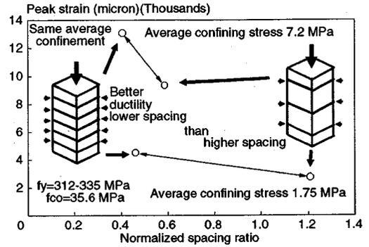
Fig.19 Peak strain under the same average confining stress
