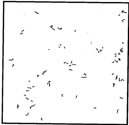
Fig.8 Microcracks on the surface of concrete (Rate of temperature rise : 12 °C /hr, Presteaming period : 4 hr, Rate of cooling : -3 °C /hr, Series 2)
