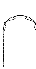
Fig. 18 Deformation of Y-Shaped Joint Elements on Soil Core (Partial Model with Joints fixed)
