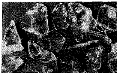
Fig.10 Micrograph of the glass grains at magnification of 10 times.
