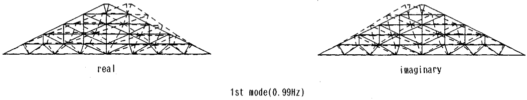
Fig. 10 Modal deformation (CASE-1).
