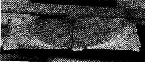
Photo 2 T-8 Specimen 1) , blowhole 0.6×0.4 mm Failure Surface with Beach Marks S=216 MPa, N_f=1.708 \times 10^3 .
