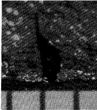
Photo 8 Small Blowholes with Fatigue Cracks (BD-1 Specimen).
