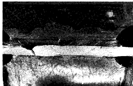
Photo 4. Crack Initiation from a crater.
