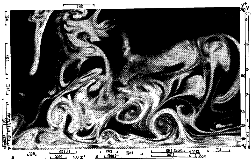
Fig. 3 Streamwise vortices in the near-wall region (CASE A).
