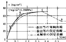
図-17  $\tau$ -S曲線
