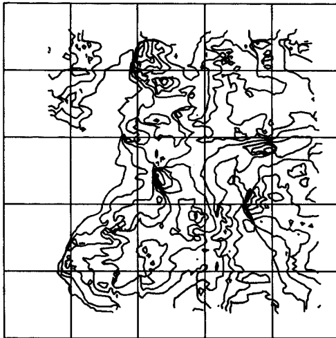
Fig. 7 Contour Map Plotted through Stereo Matching with Adaptive Search Window (c); Contour interval=20 m.
