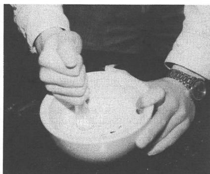
(a) Grinding diatomaceous earth into powder
