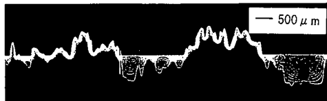
Fig.34 Fe^{2+} concentration profile of two-dimensional biofilm model with diffusion layer of 0 \mu m depth. (Run.3)
