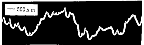
Fig.40 Fe 2+ concentration profile of biofilm model with generated rough surface from filtered spectrum by low pass filter. (Cut off frequency is 6 cycle/mm)
