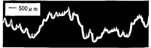
Fig.38 Fe 2+ concentration profile of biofilm model with generated rough surface from average spectrum. (Run.3)
