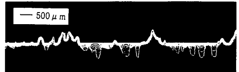
Fig.32 Fe^{2+} concentration profile of two-dimensional biofilm model with diffusion layer of 100 \mu m depth. (Run.2)
