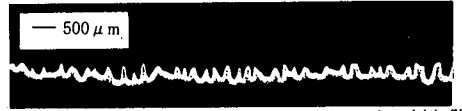
Fig.20 Fe^{2+} concentration profile of two-dimensional biofilm Model. (at lower part of reactor. Run.1)
