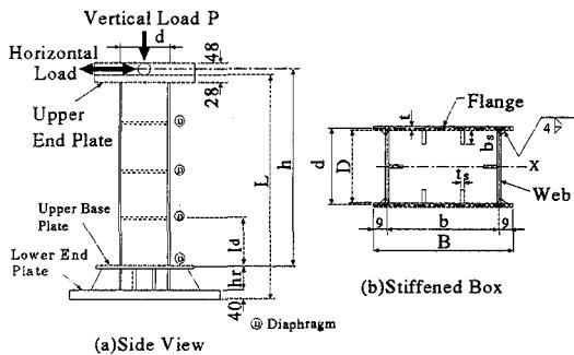
Fig.1 Test Specimen
