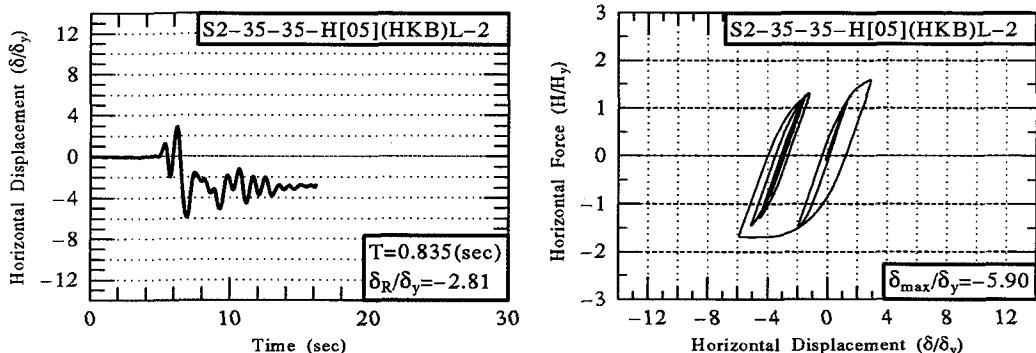
Fig.8 Response due to Amplified Higashi-Kobe (Specimen No.4)
