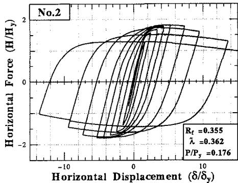
(a) Cyclic Test ( $n=1$ )
