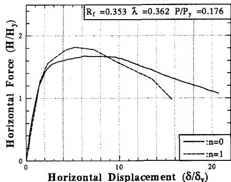
(b) Envelope of Cyclic Test ( $n=1$ ) and Monotonic Test ( $n=0$ )
