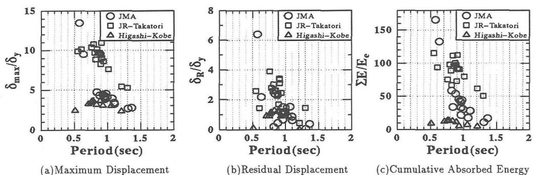
Fig.9 Maximum Displacement, Residual Displacement and Cumulative Absorbed Energy Spectra
