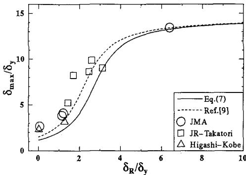
Fig.10 Comparison of Eq.(7) with Test Results
